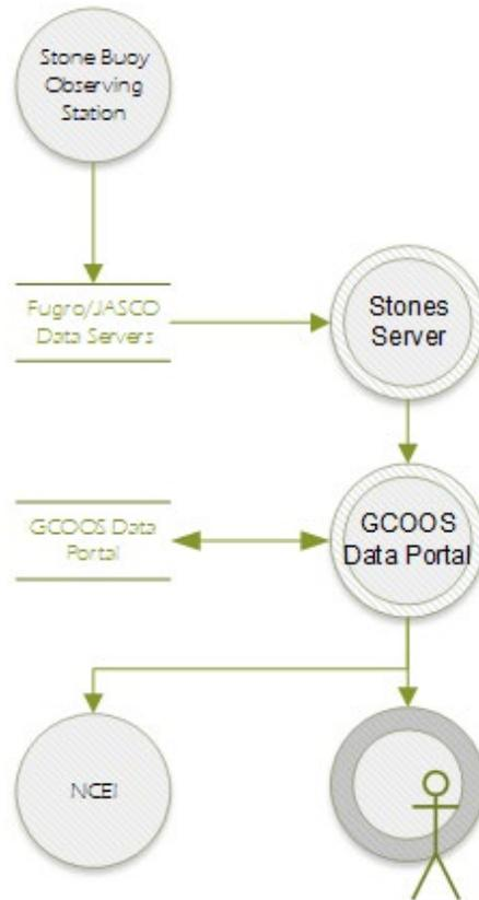
Figure 1. Data Flow Diagram of the Stones Metocean Observatory.
